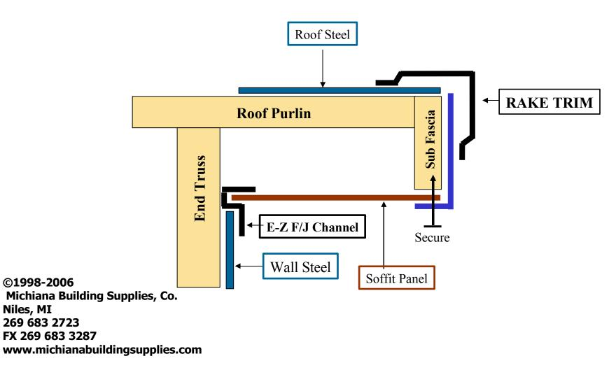
Gable End Overhang Detail- Steel Roof with /J Channel
