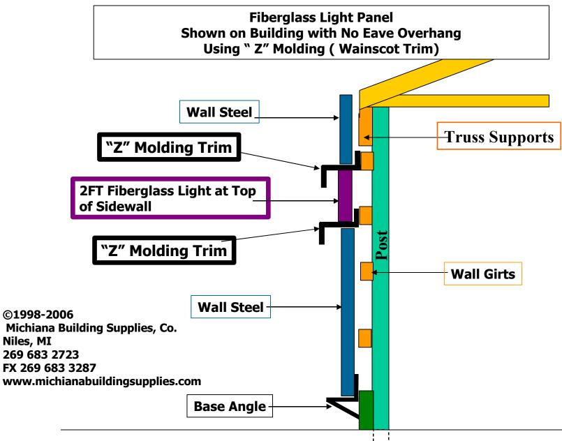
Fiberglass Light Panel Shown on Building with Eave (Sidewall ) Overhang Using " Z" Molding ( Wainscot Trim)
