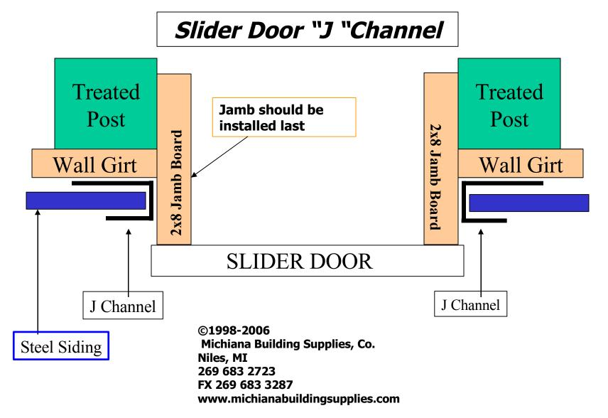
Slider Door- Basic Header and Track Board Detail
